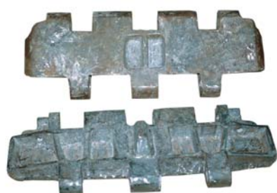
Leg-irons for bulldozers, towed grader
