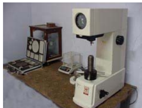
Rock well/ Mechanical testing apparatus
